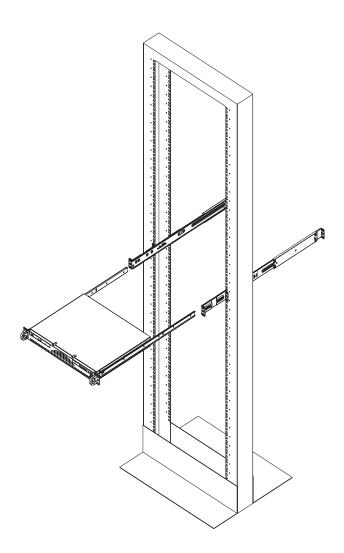
Figure 2-5. Installing the Server into a Telco Rack (w/ Optional Rackmount Kit)
